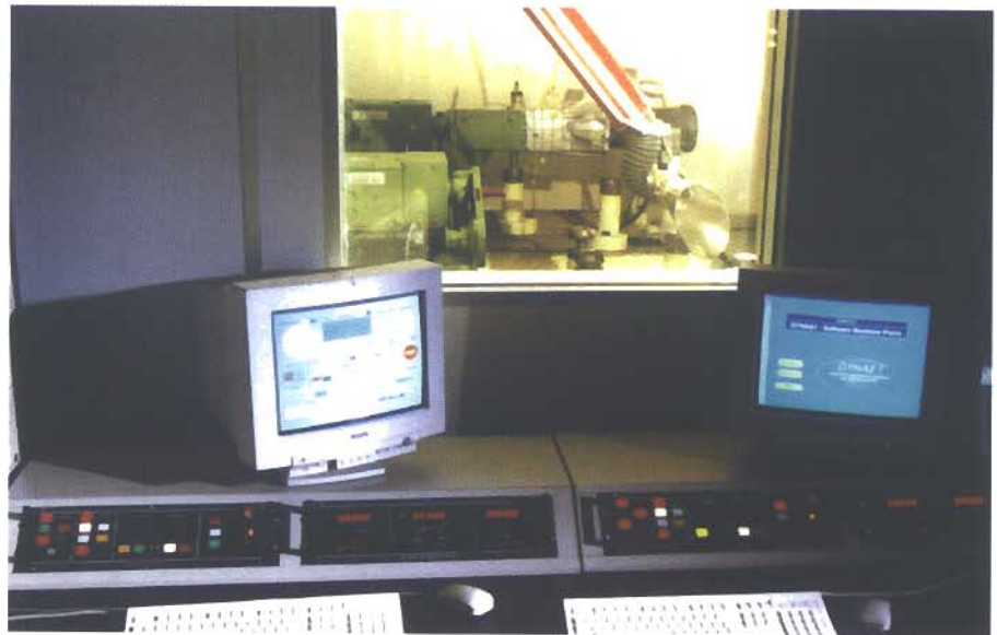
Control room; twin 30 kW brakes
