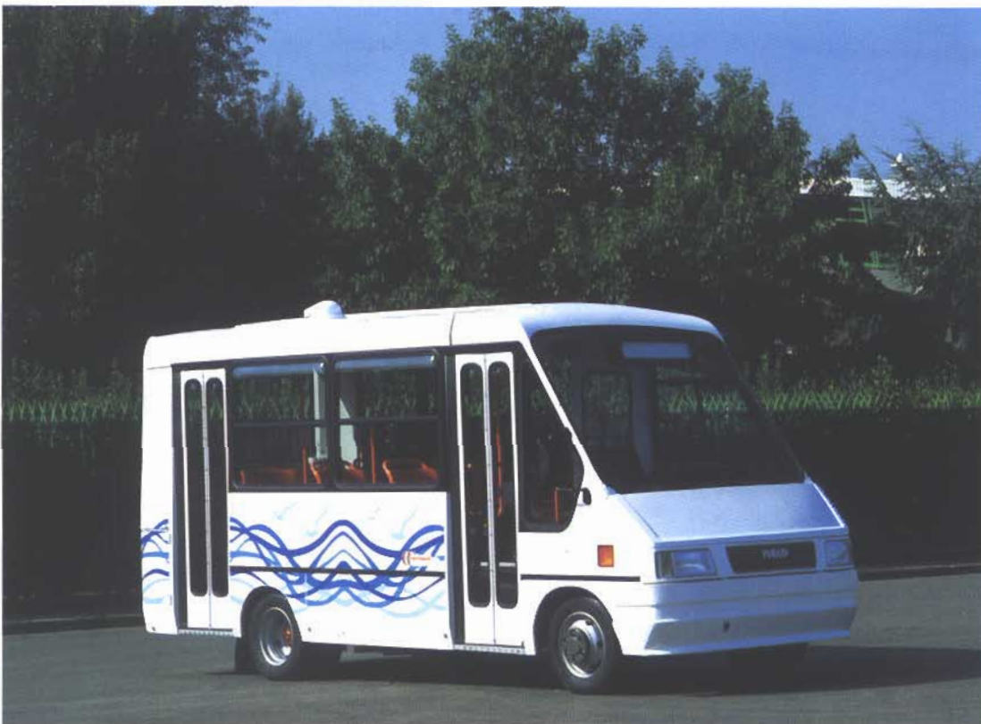
Six-metre-long hybrid mini-bus manufactured by ALTRA
